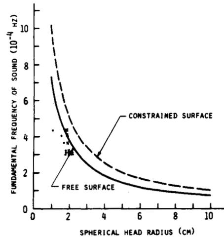
Fig. 8. Comparison of computed fundamental sound frequency and measured cochlear microphonic frequencies [20].
