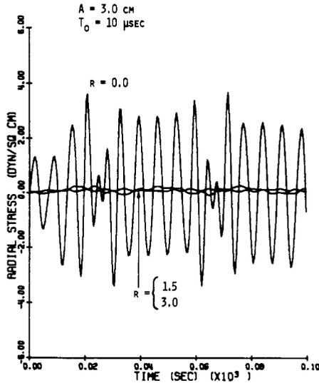
Fig. 9. Computed acoustic pressure in a spherical model of a cat-size (3-cm radius) brain exposed to 2450-MHz radiation at a SAR of 1 W/g [18].
