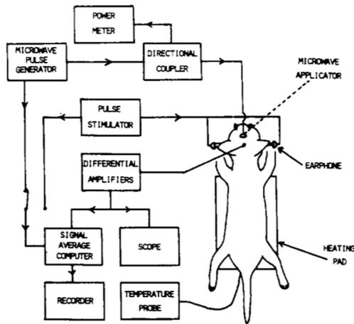
Fig. 2. Arrangement of equipment used to test microwave auditory effects in laboratory animals.
