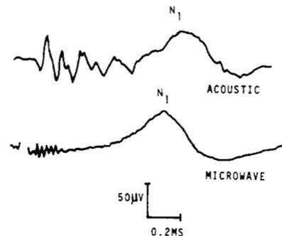
Fig. 6. Cochlear round window recording of the cat in response to acoustic and microwave pulse stimulation. Note cochlear microphonics precedings  $N_1$  responses [7].
