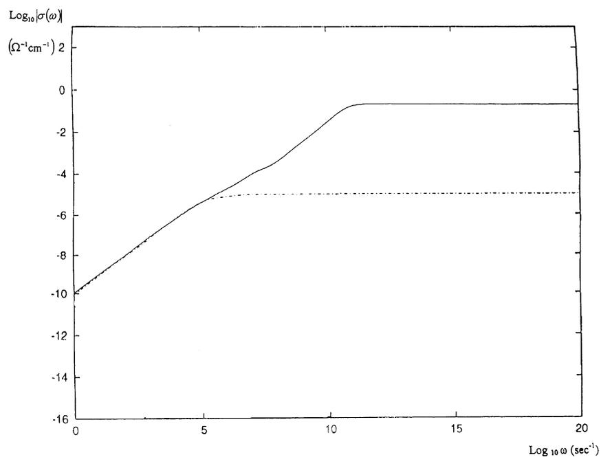
Fig. 3.  $|\sigma(\omega)|$  as a function of  $\omega$  ( $T = 298$  K).  $\omega_{\text{sat}} = 10^{10} \text{ s}^{-1}$  if 200 levels were taken into account in the valence bands region (—) and  $\omega_{\text{sat}} = 10^5 \text{ s}^{-1}$  if only 100 levels were considered. (- - -).
